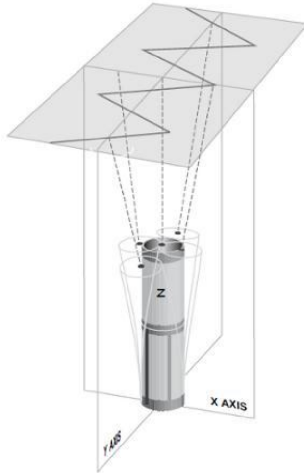
Figure 1: Raster pattern created by the piezoelectric scanner. The y-direction is the slow scan direction and the x-direction is the fast scan direction. Image credit: Bruker Nanoscope Software (v8.10r2) Manual.
